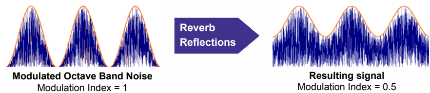
Figure 6: Reverberation, background noise and reflection are responsible for degrading of the modulation index.
